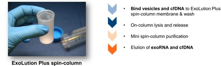
**Workflow for co-isolation of exoRNA and cfDNA from biofluids using the ExoLution Plus technology platform.** The ExoLution Plus platform employs a proprietary capture mechanism in a disposable spin-column format to enable routine parallel co-extraction of exoRNA and cfDNA from biofluids.
