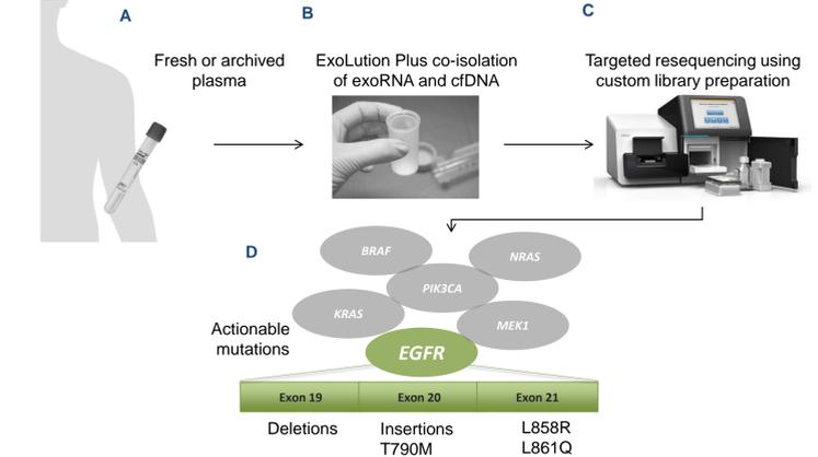
**Workflow of the ExoDx Solid Tumor Panel:** ExoLution Plus co-isolation of exoRNA and cfDNA from 0.5-4 mL of fresh or archived plasma, pre-filtered to exclude cellular material (A and B); Targeted enrichment, sequencing on the Illumina MiSeq™ platform of input material; Bioinformatics analysis including noise reduction and mutation calling (C and D).
